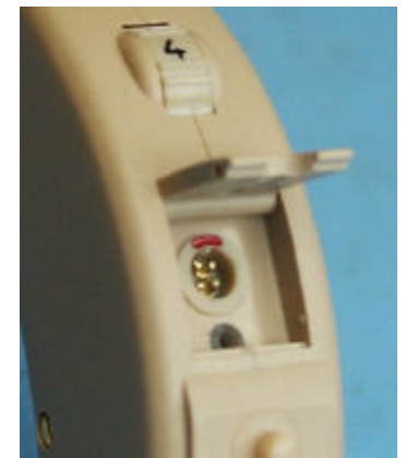
Concealed Programming Socket and Rear Directional Microphone
