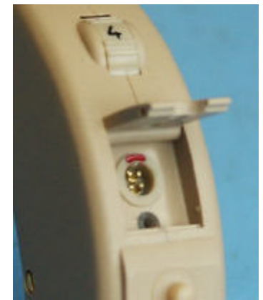
Concealed Programming Socket and Rear Directional Microphone
