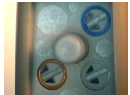
Three Trimmers allow for greater flexibility. Push Button enables the powerful Telecoil.
